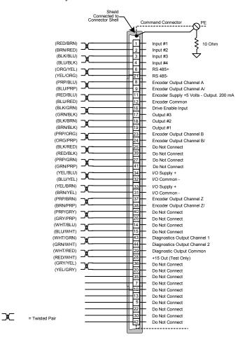
(ECI-44) which provides a convenient screw terminal connection strip. Connect one end of the CMDX command cable to your drive and the other end to the ECI-44.
